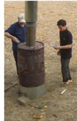
Reducing Temperature to about 450- 550C with spray water
