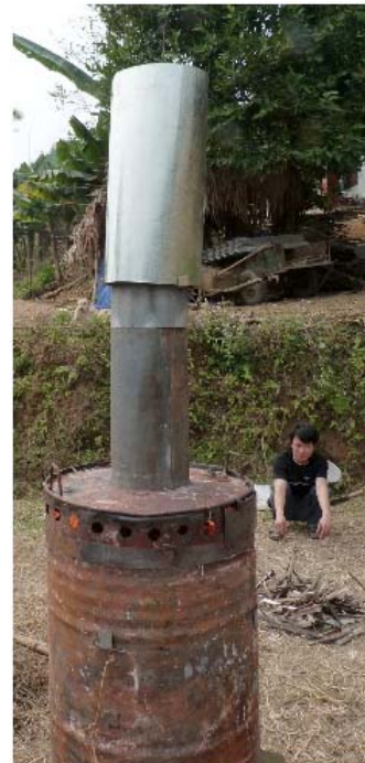
TLUD drum oven operating in a rice paddy
